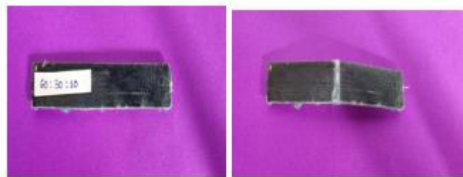
Fig. 10. Specimen 1 before and after bending test
