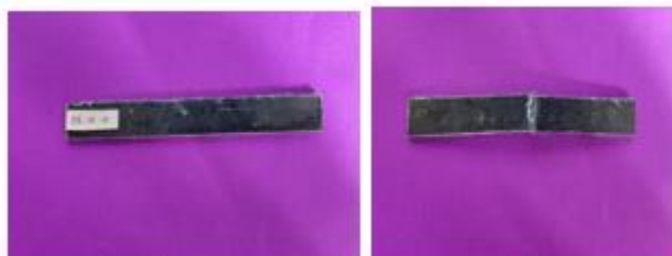
Fig. 8. Specimens 2 before and after tensile test
