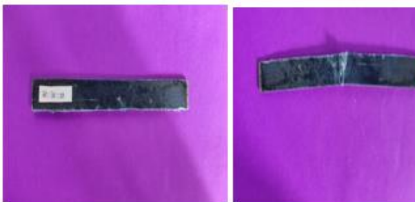
Fig. 6 Specimens 1 before and after tensile test
